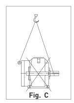
Don't lift units with slings wrapped around shaft (See Fig. c). Gear units with forced lubricants system should be handling with care to prevent damage to the pumps & pipe lines.
