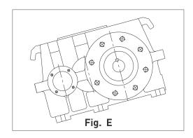
The gear units fix on its foundation with proper bolts size. Tightening of bolts must be done properly with torque wrenches to avoid over stressing of the bolts.
